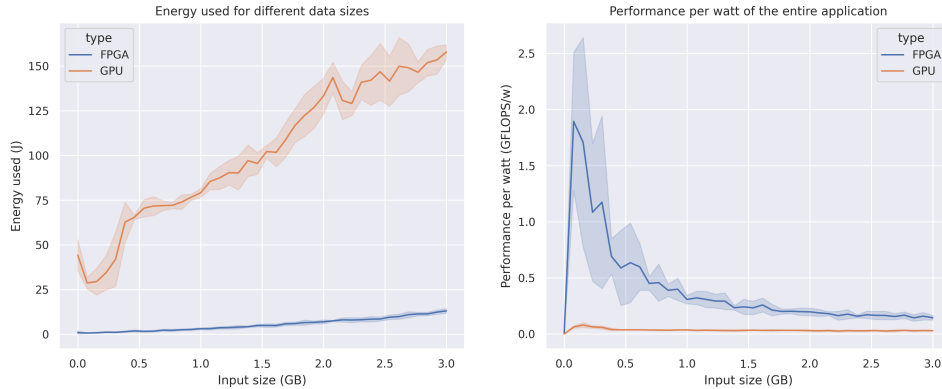
Figure 4.8: Energy consumption of the vector addition applications of the GPU and FPGA
