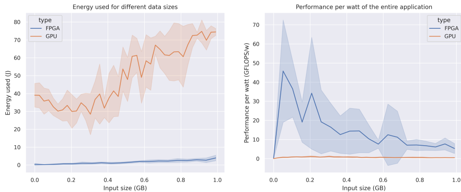
Figure 5.7: The energy consumption of the FPGA and GPU for the 5-point stencil computation
