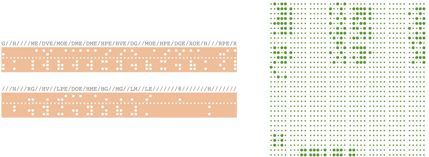
The program is in the top half of the tube, in two columns, and the variables are at the bottom. The input  $n = 10 = 1010_2$  is in line 29, while the output  $u = 10! = 110111010111110000000_2$  is in line 30.
