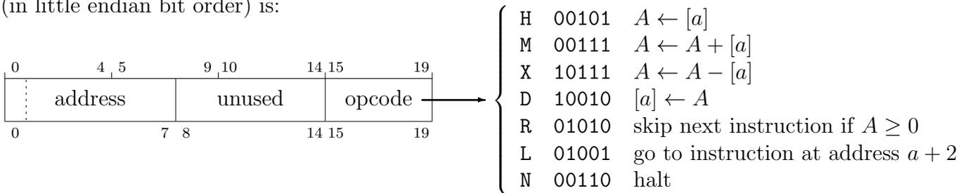
In this  $A$  is the accumulator,  $a$  is the address, and  $[a]$  the 40-bit word at that address in memory. After an instruction is executed, the program counter (where the lower bit is *not* ignored) is increased by *two*, so execution will proceed on the same side on the tube.
