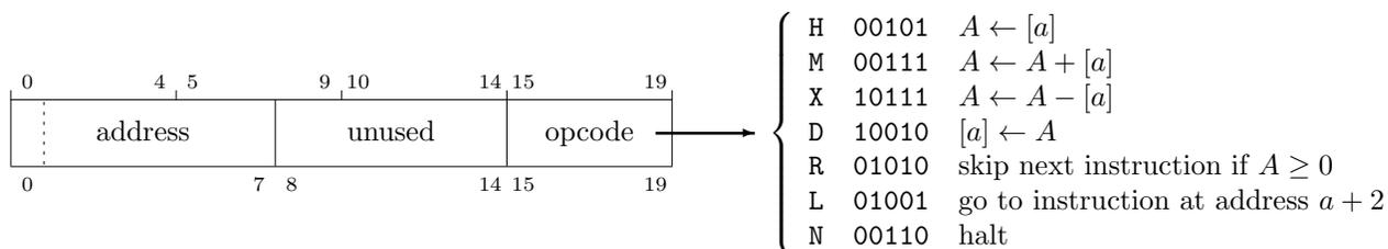
In this,  $A$  is the accumulator,  $a$  is the address, and  $[a]$  the 40-bit word at that address in memory. After an instruction is executed, the program counter (where the lower bit is *not* ignored) is increased by *two*, so execution will proceed on the same side on the tube.
