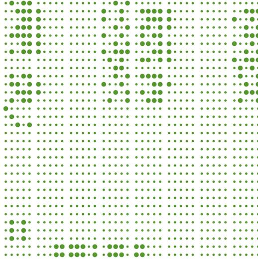
The program is in the top half of the tube, in two columns, and the variables are at the bottom. The input  $n = 10 = 1010_2$  is in line 29, while the output  $u = 10! = 1101110101111100000000_2$  is in line 30.
