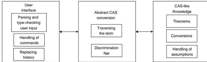
**Fig. 1.** Architecture of a CAS inside a TP system with responsibilities of the parts of our implementation marked. The prover is not marked on the figure, since all parts make use of it, by using its type of terms and theorems, as well as tactics and conversions to build them.
