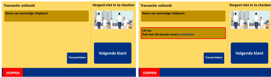
Figure 5.10: Check in warning - old and new
