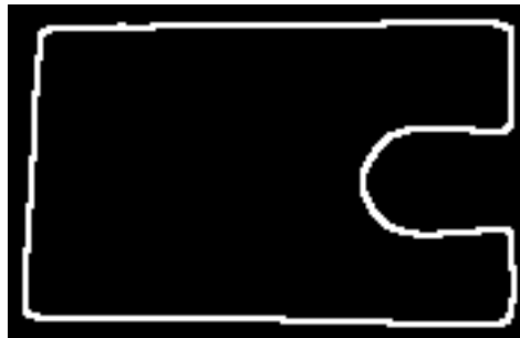
Fig. 4.2: An edge-detected business card, distorted by a thumb holding it.
