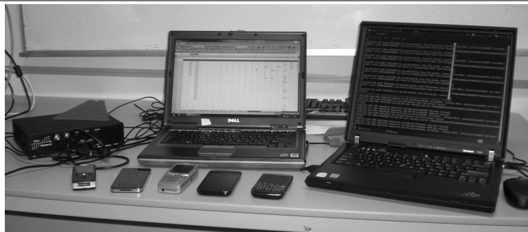
Figure F.2 The setup with on the left the USRP-1, on the right the notebook running OpenBTS and in the centre the notebook used for bookkeeping. In the front are five cell phones.
