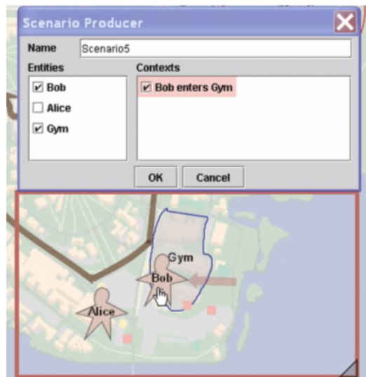
Figure B.7: A dialog box is then brought up that lets designers select contexts of interest. The left side of this dialog box contains a list of entities that can be used for filtering contexts. Unchecking an entity removes all contexts associated with that entity.
