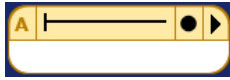
Figure A.2: An orange prompt card is used to indicate a system prompt, something the computer says to the user. You can add a prompt card to your design by either clicking your right mouse button in the canvas area or by dragging a card from the script bar. (The script bar is covered in detail in section 2.) Prompt cards are moved in the same way as the start card: by right-clicking over it and dragging it around.
