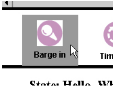
Figure A.17: In the Wizard options bar you have the option to select barge-in. Barging-in is when the user begins giving his or her response before the prompt is done playing. If the user does this, you can click the "barge-in" button and SUEDE will stop the prompt from playing and will immediately start recording.
