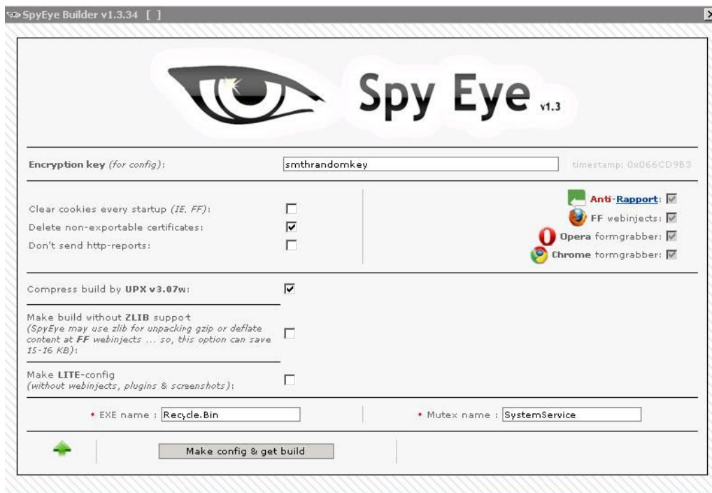
Figure 2.5 A screen shot of a Spyeye binary builder. This will build a fresh version of Spyeye for this owner, to help prevent detection.
