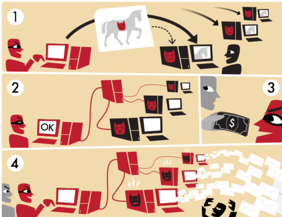
Figure 4.2 The stages of a botnet infection, an illustration of how a compromised system might be used to send spam [Wikipedia http://en.wikipedia.org/wiki/File:Botnet.svg ]
