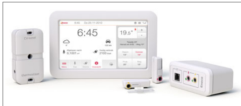
Figure 3: The Toon HEMS. From left to right: the central heating module (not discussed in this thesis), the IHD, the two sensors for gas and electricity meters, and the gateway.
