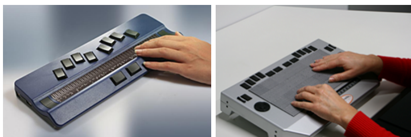
Figure 4.4.: Active Braille refreshable braille display and Hyperbraille tablet.
