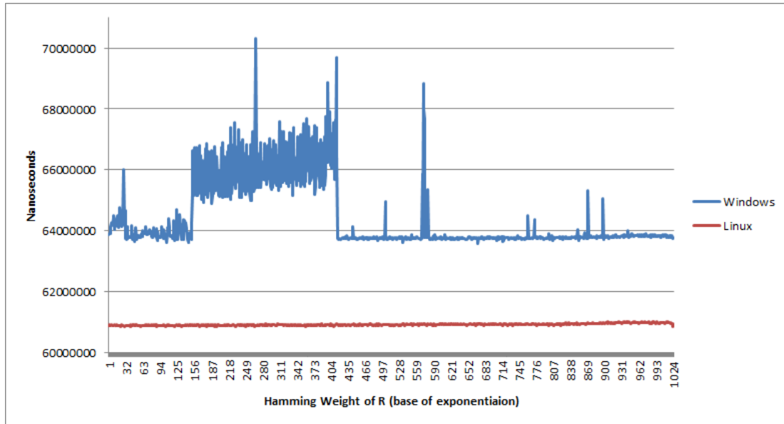
Figure 7.4: Average execution times based on 1250 runs per Hamming weight value for the base of the exponentiation ( R ).
