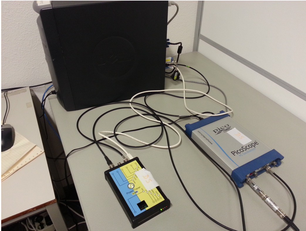
Figure 3.1: Set-up that was used for the acquisition of the power traces of the smart card.
