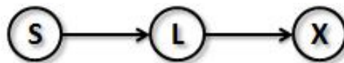
Figure 3 - Head-tail: variable S and variable X are conditionally independent given variable L
