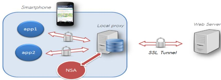
FIGURE 4.1: NSA application architecture: HTTP traffic is intercepted by a local proxy service
