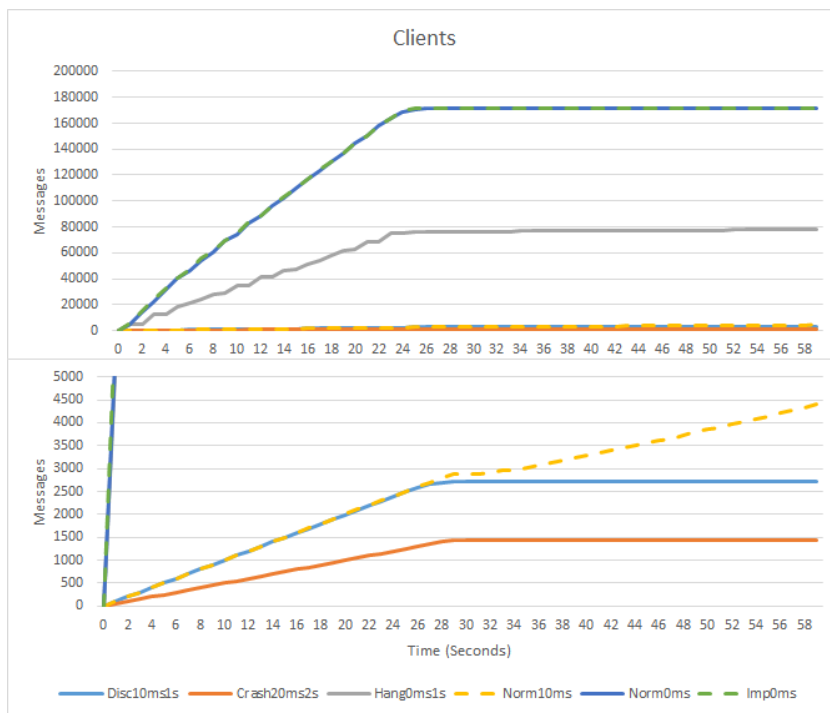
Figure 12: WithObserveOn for nonessential subscriber; Null solution for essential subscriber.
