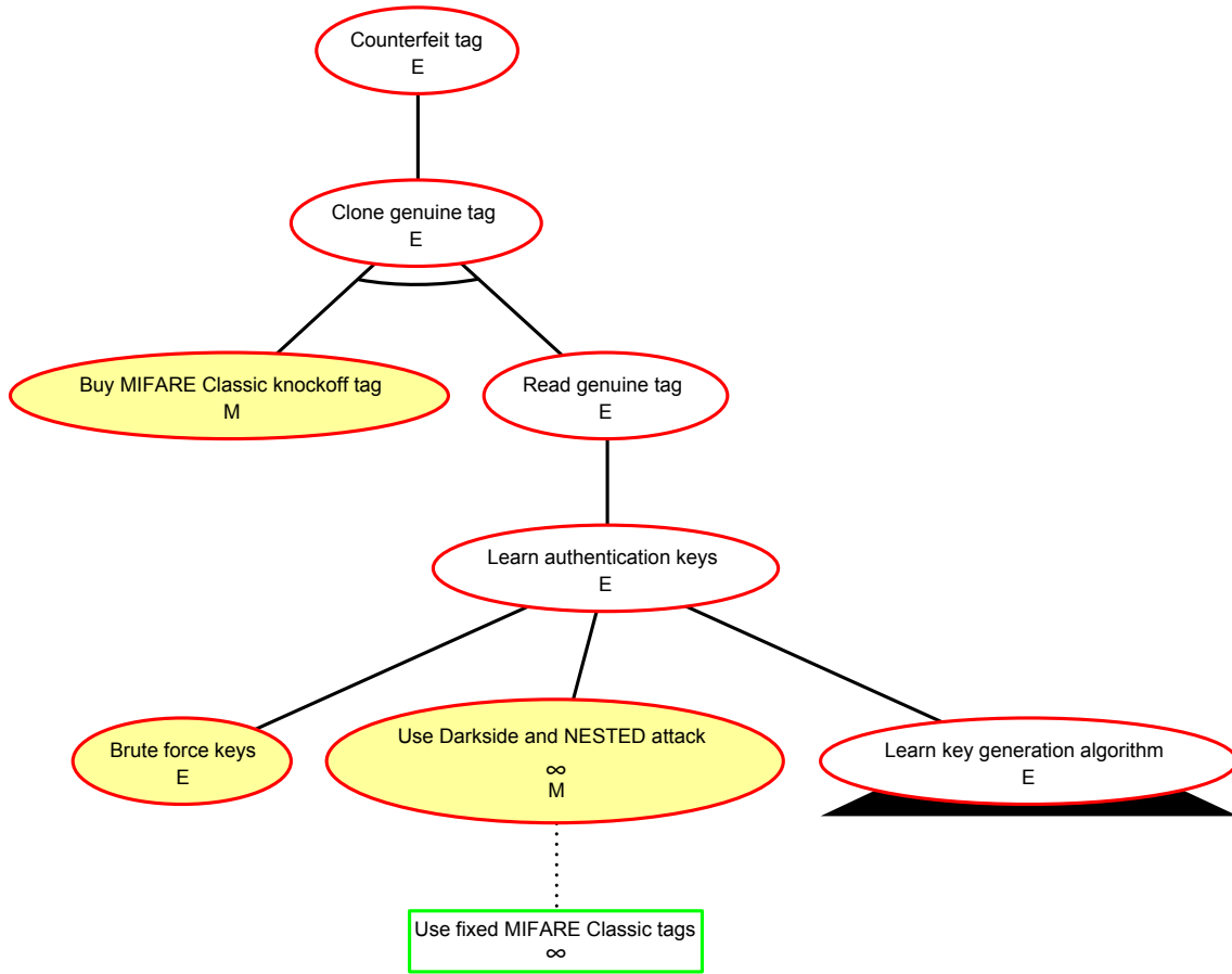
Figure 4: Attack-defense tree to clone a genuine tag using the minimal difficulty level attribute domain \{\text{Low}, \text{Medium}, \text{High}, \text{Extreme}, \infty\} , see Figure 7 for the Learn key generation algorithm tree.
