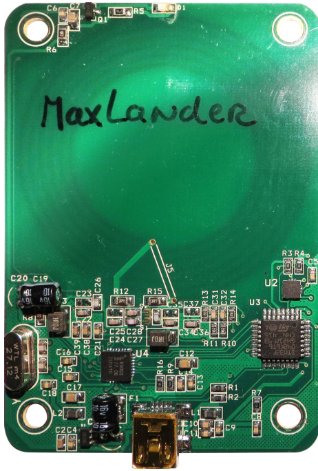
Figure 31: Front of the MaxLander PCB, "SAM12" is printed on the U2 IC
