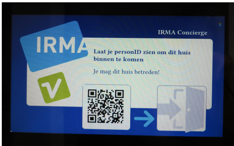
Figure 6.10: If there is a matching house rule containing the revealed personID attribute, then this screen will be displayed and the door will be opened.
