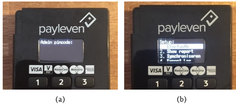
Figure 6.4: The admin menu. (a) The card reader prompts for the admin PIN. (b) The upper menu items (4 items).
