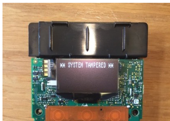
Figure 6.3: The message on the display indicates that the card reader has been tampered with.
