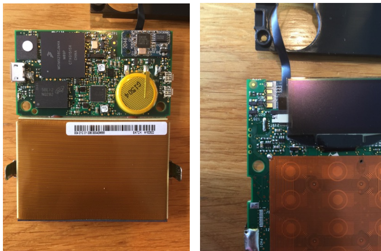
(a) The internals of the card reader demonstrating the integrated circuit. (b) The magnetic strip reader is loosened from the card reader.
