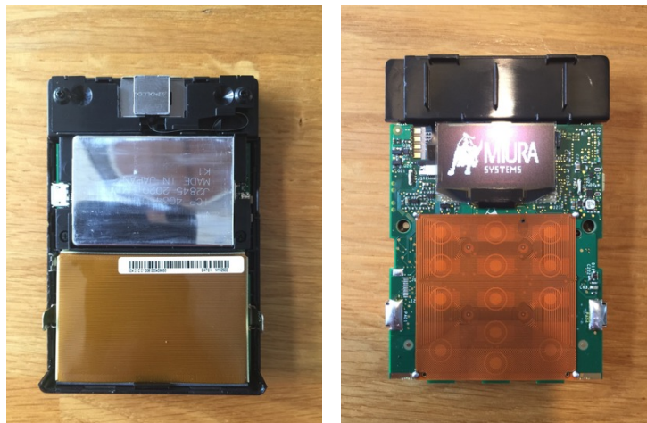
(a) The backside of the card reader without plastic casing. (b) The frontside of the card reader without plastic casing.
