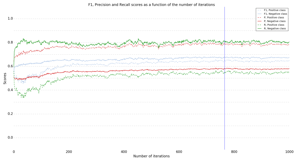
(a) F_1 , precision and recall scores for both classes as a function of the number of iterations. The blue vertical line marks the best F_1 score for the negative class.
