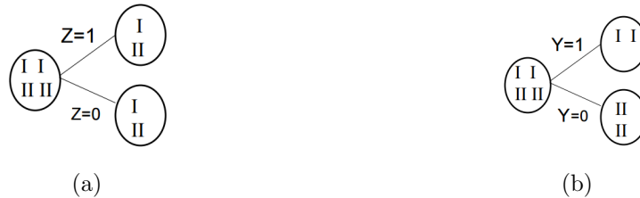
Figure 2.2: Examples of (a) no gain and (b) gain, while using Information Gain
