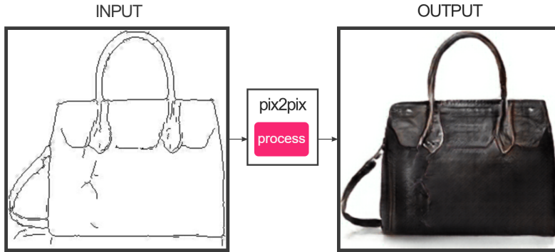
Figure 3.10: Translation of an image with the Pix2Pix GAN [31]. The Pix2Pix GAN gets an input image from some domain and learns to map that to a different domain. In this example, the drawing of the handbag is mapped to a realistic image of a handbag.
