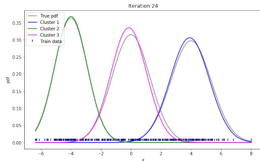
Figure 4.2: Three Gaussians fitted to the sampled data gives us three almost identical Gaussians. If this were modeled using a single Gaussian, sampled data would be very different than the real data. From [4].
