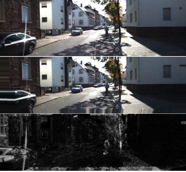
Figure 5: Example of the photometric error Top: The reconstruction target image. Middle: Reconstruction made from the next video frame. Bottom: The calculated photometric error between the target and the reconstruction.
