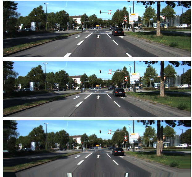
Figure 1: Effects of occlusion on the reconstructed image. Top: The image for which the depth prediction is made. Middle: The next video frame, captured 100ms later. Bottom: Reconstruction of the first image made by sampling from the next video frame. The lane markings at the bottom of the image are incorrectly reconstructed because they are not visible in the next frame. The tree on the right-hand side of the road appears twice in this reconstruction. This happens when areas with different predicted depths are projected to the same area. In other words, the sampling would have been correct if the tree was not blocking the view.
