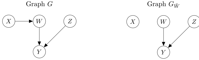
Figure 2.6: Example in which rule 1 applies. We can see that X and Y are d-separated by W and Z in graph G_{\bar{W}} .
