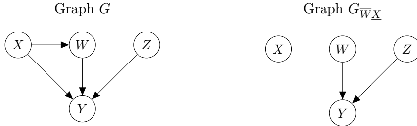
Figure 2.7: Example in which rule 2 applies. We can see that X and Y are d-separated by W and Z in graph G_{\bar{W}\underline{X}} .
