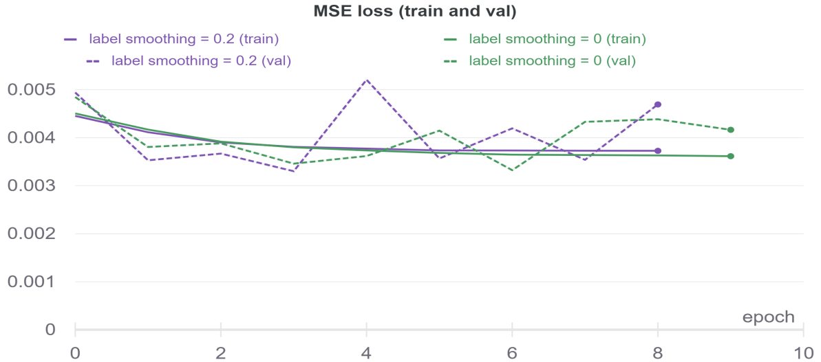
Figure A.3: Performance when using label smoothing (label smoothing factor of 0.2) versus no label smoothing at all (label smoothing factor of 0). Note that the MSE is not terms of mm/h but it is calculated on the normalized dBZ values. The models were run for 10 epochs with early stopping after 5 epochs of no improvement.
