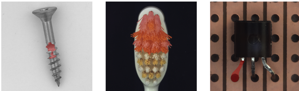
Figure 4.1: An example of a screw, toothbrush and transistor that are defective.
