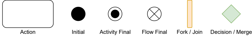
Figure 2.11: Basic constructs of a SysML activity diagram considered in the Activity Calculus.
