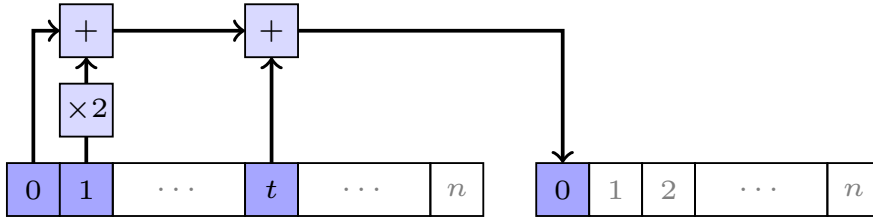
Figure 4: A schematic overview of the \theta operation with c_0 = 1 , c_1 = 2 , c_t = 1 and all other c_j = 0 using the one-dimensional representation. Here, it is shown that the state digit s_0 is adapted by \theta resulting in the state digit \theta(s_0) . In the figure the state digits s_i are denoted as i .
